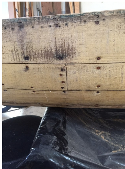
Cedar planking, with steel boat nails. RC Cross photo
