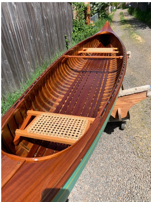
Caned seats replaced the woven steel strapping seats, which might not have been original. RC Cross photo
